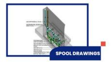
A pipe spool drawing is optimized to provide all the information needed by the fabricator to accurately manufacture or assemble the spool. Spool drawing furnishes the complete information of all parts welded together in the shop on a single drawing.
