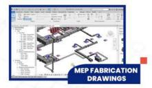
A step on from installation drawings are fabrication drawings. We have often produced fabrication drawings from our coordinated ductwork model. When doing these drawings we liaise with the ductwork fabricator to ascertain their standard manufacturing dimensions such as cut-length and gasket thickness.
